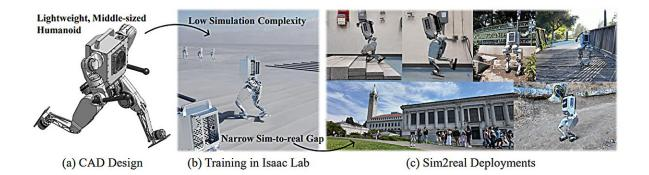
Design, training, and sim-to-real deployment of our custom-built humanoid with a learning-based controller. Credit: *arXiv* (2024). DOI: 10.48550/arxiv.2407.21781
