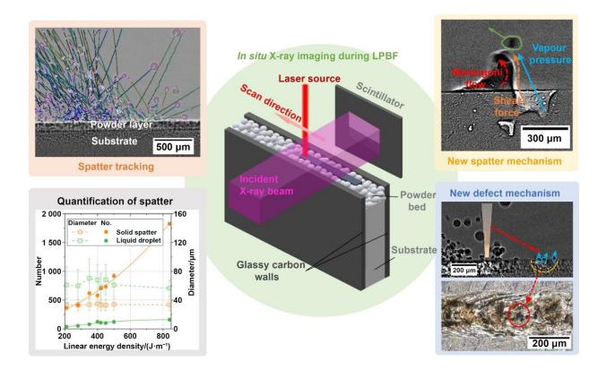
Through high-speed synchrotron X-ray imaging, the spatter dynamic during LPBF was captured and quantified under various processing conditions, and two new spatter mechanisms were discovered. Credit: Da Guo, Rubén Lambert-Garcia, Samy Hocine, Xianqiang Fan, Henry Greenhalgh, Ravi Shahani, Marta Majkut, Alexander Rack, Peter D Lee and Chu Lun Alex Leung.
