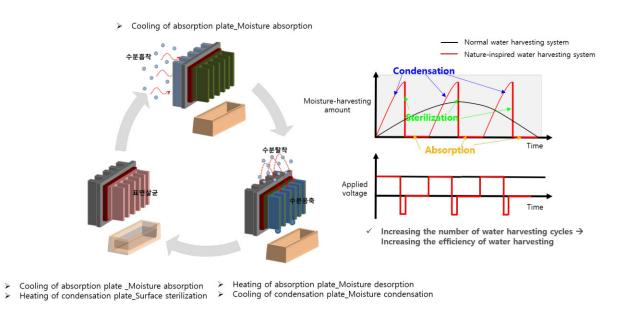
Concept of the core technology for the moisture collection cycle to increase moisture collection and energy efficiency. Credit: Korea Institute of Machinery and Materials (KIMM)
