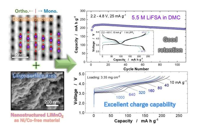
Nanostructured  $LiMnO_2$  with domain structures and larger surface area delivers large reversible capacity with good capacity retention with excellent charge rate-capability, which is an essential character for electric vehicle applications. Credit: Yokohama National University
