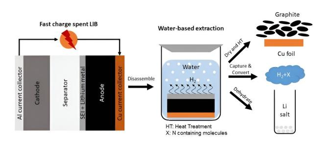
Process overview, left to right: Fast charge of the lithium-ion battery. Disassemble battery into individual parts. Place components in water and add  $CO_2$ . Use various processes to recover materials from the battery components. Credit: Ames National Laboratory
