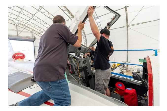
Lockheed Martin technicians temporarily remove the canopy from the X-59 in preparation for final installation of the ejection seat into the aircraft. Credit: Lockheed Martin
