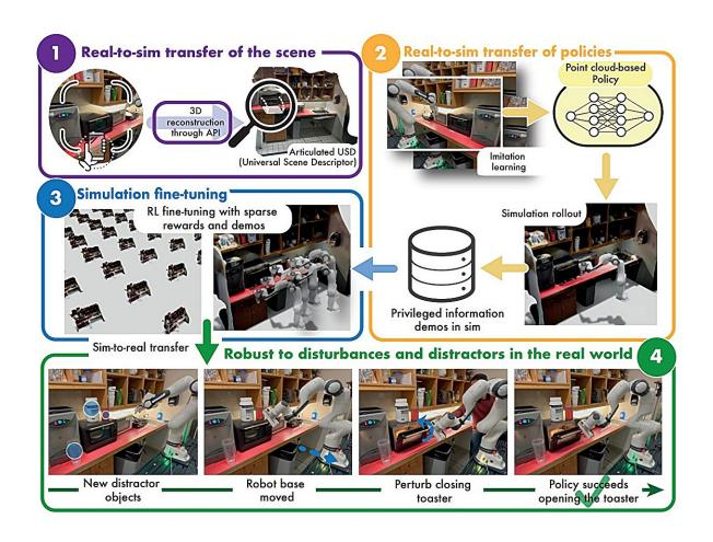
RialTo system overview. 1) Transfer the real-world scene to the simulator through an easy-to-use API (see Section III-B). 2) Transfer a policy learned from real-world demonstrations to collect a set of demonstrations with privileged information in simulation. We note this step is optional, and RialTo is
