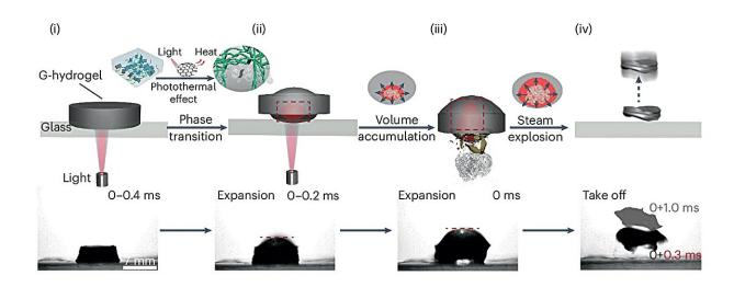
Schematic of the ASEF mechanism and high-speed camera images showing the take-off from a glass substrate. Credit: *Nature Materials* (2024). DOI: 10.1038/s41563-024-01955-4
