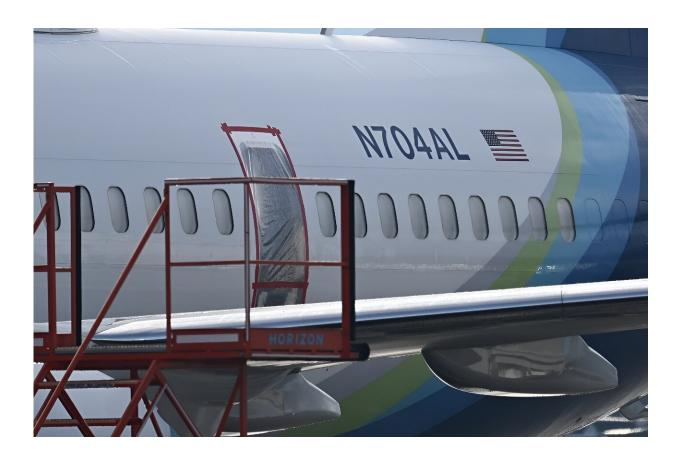
A two-day hearing is set to investigate what happened on a January 5 Alaska Airlines flight in which a panel on the fuselage of a 737 MAX blew out mid-flight.
