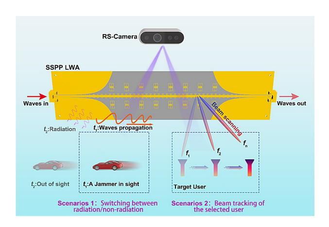
Schematic of the smart SSPP-LWA system. The RS-camera automatically detects the moving target—a model car or a target user in the environment. The position information of the target is sent to the control system, the supply voltage (via a FPGA) or input power (via a signal generator) is fed back in a few milliseconds, and the working status of SSPP-LWA is altered or the beam tracking are realized accordingly. Credit: OES
