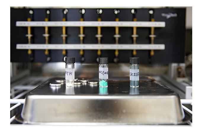
SKIER-5 developed through the oxidation reaction of trianthrene and nickel ions (from left to right trianthrene, nickel, SKIER-5). Credit: Korea Institute Of Energy Research
