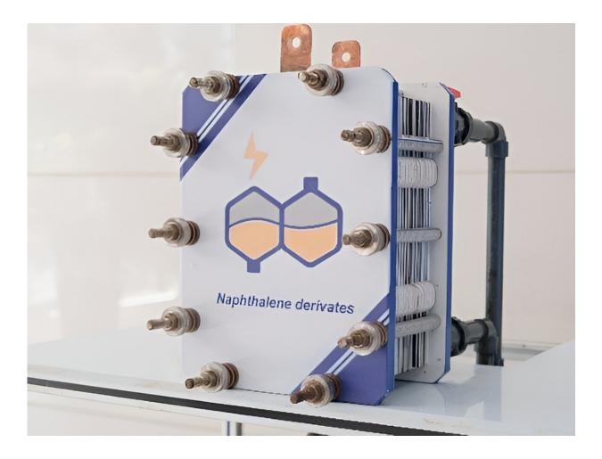
A pilot-scale naphthalene-based flow stack. Credit: DICP
