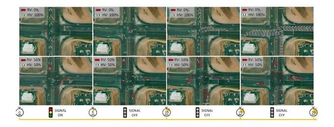
Simulating a blackout at a traffic intersection. The top row shows traffic conditions without robovehicles. The blackout occurs at the 5-minute mark. Congestion forms rapidly within 15 minutes. The bottom row shows traffic with 50% robovehicles. The blackout causes no congestion. Credit: Wang et al
