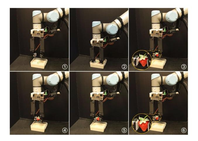
In-hand singulation manipulation involves rubbing off residual rice from between the finger and the grasped artificial strawberry. Credit: Zhou et al.
