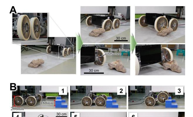
Evaluation of wheel characteristics based on the surface tension. Credit: Sung-Hyuk Song, Korea Institute of Machinery and Materials
