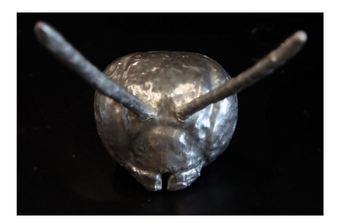
Metallic replica of a honeybee's (Apis mellifera) head, created at room temperature and pressure, using the same principles insects use to form their exoskeleton. Credit: SUTD
