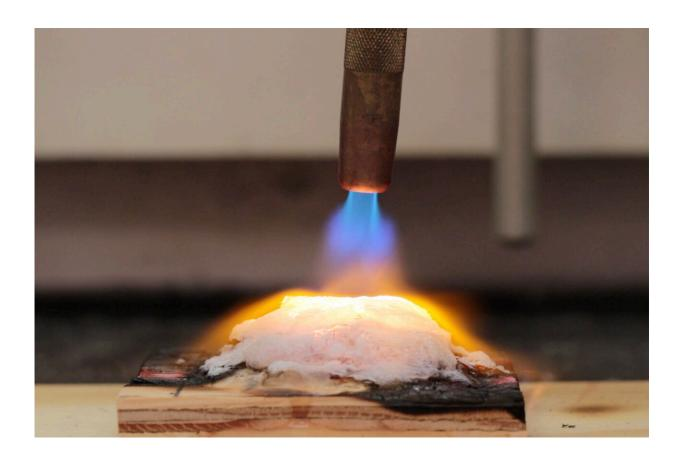
During a test on plywood, researchers showed how the new gel transitions from a hydrogel to an aerogel under heat from a gas hand-torch. The torch burned at a much higher temperature than would result from a wildfire. Credit: Andrea d'Aquino
