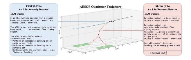
Closed-loop trajectory of a quadrotor using the AESOP algorithm. Credit: *arXiv* (2024). DOI: 10.48550/arxiv.2407.08735
