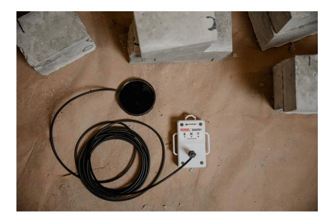
From beneath a concrete pour, this black circular sensor transmits data about concrete strength levels through a cord plugged into an aboveground device called a data logger. Engineers receive real-time data from this device through an app. Credit: Purdue University /Greta Bell
