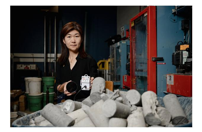
Purdue University professor Luna Lu holds the REBEL concrete strength sensing system, which her lab invented to improve estimates of in-place strength of concrete structures. As a beta product of Wavelogix, founded by Lu, the REBEL sensor technology is being tested in several states. Credit: Purdue
