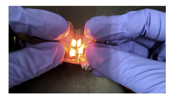
Researchers have developed a technique for printing thin metal oxide films at room temperature, and demonstrated the technique by printing metal oxides onto a polymer, creating highly flexible circuits. Credit: Minsik Kong
