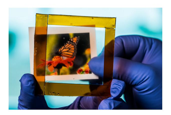
Photo viewed through a piece of glass treated with a thermochromic blend. Credit: Jeff Fitlow/Rice University.
