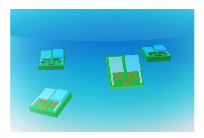
The zinc-air battery is 0.1 millimeters long and 0.02 millimeters thick. Credit: Massachusetts Institute of Technology
