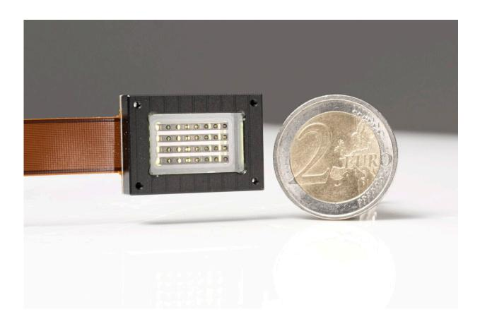
Transparent OLED microdisplay device Credit: Fraunhofer IPMS
