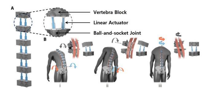
Multi-directional back support and motion assist mechanism of the BBEX. Credit: *Science Robotics*
