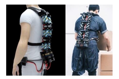
Design of the BBEX worn on a human user (left) and demonstration of weight lifting using the actual prototype (right). Credit: Seoul National University College of Engineering
