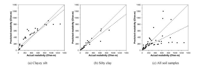
The study shows that a combination of water content, plasticity index, and dry density, can provide a reliable prediction model for soil resistivity, paving the way for the cost-effective design of reliable power grounding systems. Credit: Shinya Inazumi from SIT, Japan
