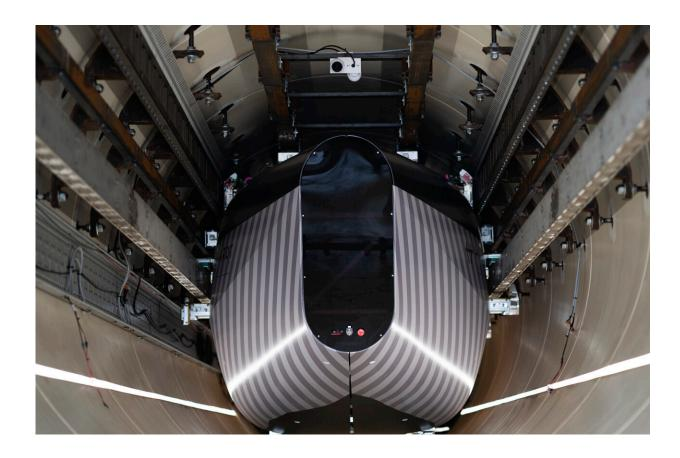
A test vehicle levitated by magnetic fields zips through a depressurized tube in a testing ground for a high-speed transit system during a press tour of an European test center for hyperloop transportation technology in Veendam, northern Netherlands, Friday, Sept. 6, 2024. Credit: AP Photo/Peter Dejong
