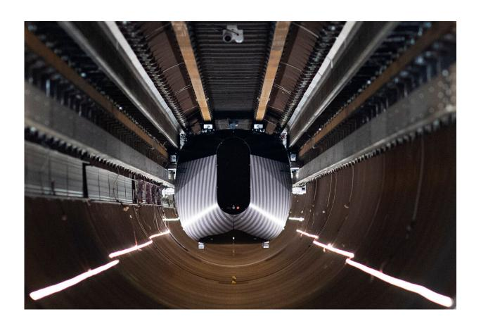
A test vehicle levitated by magnetic fields zips through a depressurized tube in a testing ground for a high-speed transit system during a press tour of a European test center for hyperloop transportation technology in Veendam, northern Netherlands, Friday, Sept. 6, 2024. Credit: AP Photo/Peter Dejong
