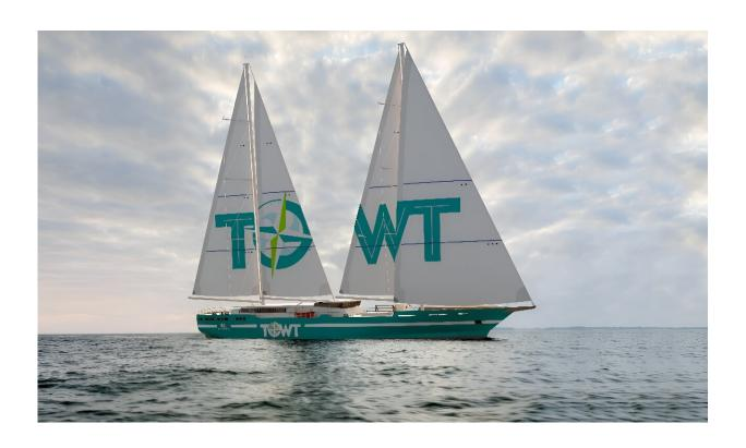
A 3D view of a prototype of the first cargo sailboat operated by TOWT.
