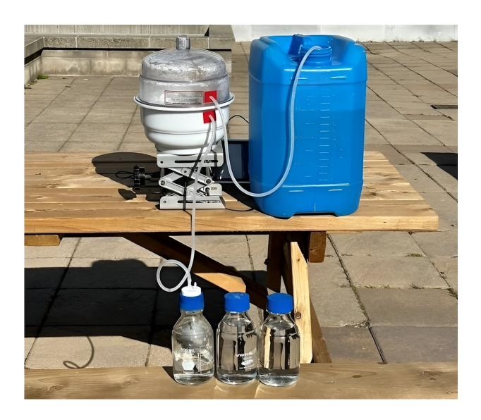
Mock-up of solar desalination system. Credit: *Nature Communications* (2024). DOI: 10.1038/s41467-024-50279-z
