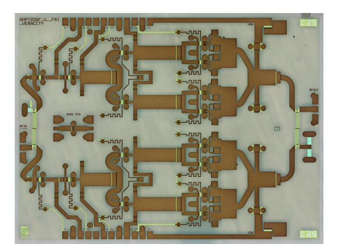
GaN amplifier circuit for inter-satellite communication links in the V-band (here: 57–70 GHz). Credit: Fraunhofer IAF
