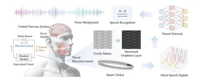
An overview of the wearable SSI, featuring an ultrasensitive strain sensor and a neural network for efficient speech recognition. Credit: University of Cambridge
