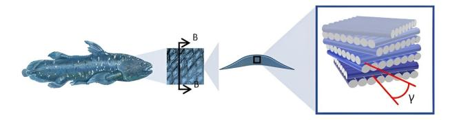
Inspired by the ancient coelacanth fish, the researchers used a strand-by-strand, double twisting architecture to enhance the concrete's toughness. Credit: Princeton University
