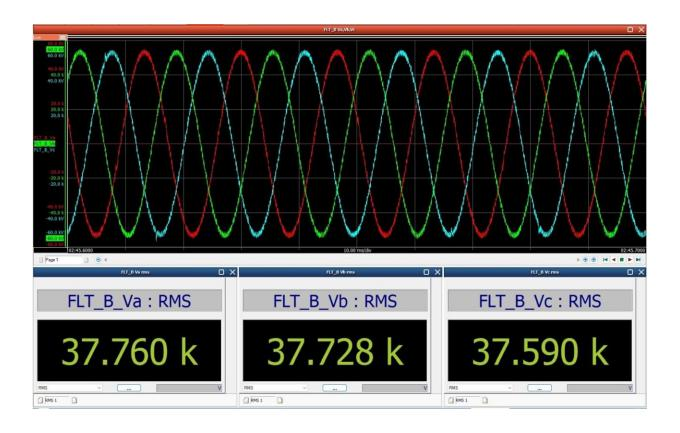
The analysis software displays measurements for the operation of the test bench under no-load conditions. The voltage values (line-to-neutral) at the simulator's output during 66 kV operation are shown. Credit: Fraunhofer IWES
