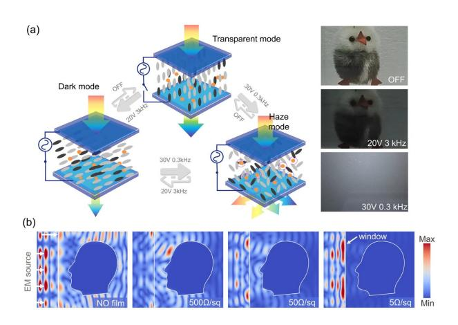
Fig. 1. a, Schematic diagram of different mode dimming control strategies and effects for the tri-state switching multispectral smart window. b, Electric field analysis of the human head behind the window with different resistance values at 5 GHz wave incidence. Credit: *Light: Science & Applications* (2024). DOI: 10.1038/s41377-024-01541-y
