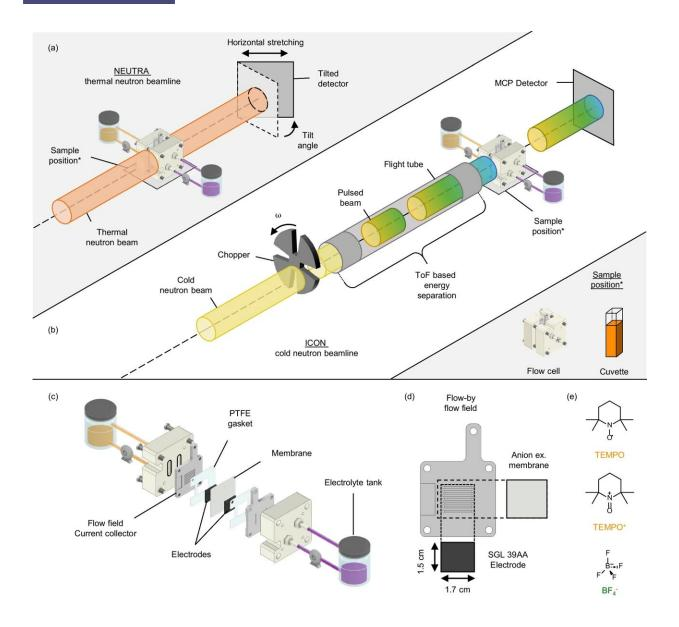
Illustration of the neutron radiography approach showing the neutron imaging setups and cell components. Credit: *Nature Communications* (2024). DOI: 10.1038/s41467-024-50120-7
