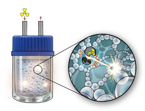
The scintillating aerogel is inserted into a scintillation vial. The gas to be analysed penetrates the vial and the aerogel via diffusion. Each decay emits an electron that interacts at very short distance with the "scintillating" nanoparticles that make up the aerogel. This results in a flash of light that is then detected, signalling the presence of the radionuclide. Credit: Zoé Dujardin
