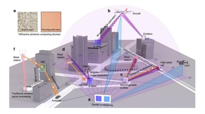
S-DNN for all-optical wireless sensing and communication. Credit: *Light: Science & Applications* (2024). DOI: 10.1038/s41377-024-01511-4
