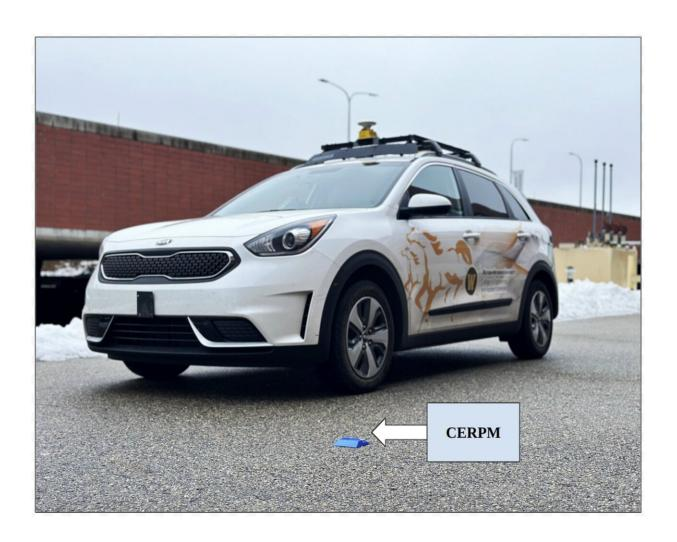
Energy-efficient autonomous vehicle (EEAV) research platform along with an RSU CERPM unit pictured at Western Michigan University. Credit: *Sensors* (2024). DOI: 10.3390/s24072327
