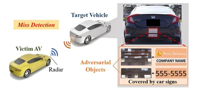
UB researchers used 3D printers and metal foils to fabricate objects in specific geometric shapes that could be strategically placed on a vehicle to make it disappear from radar detection. Credit: University at Buffalo
