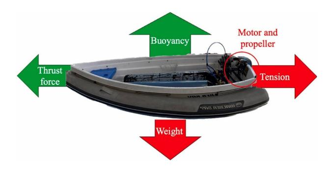
Free body diagram of the system. Credit: *Ocean Engineering* (2024). DOI: 10.1016/j.oceaneng.2024.118335
