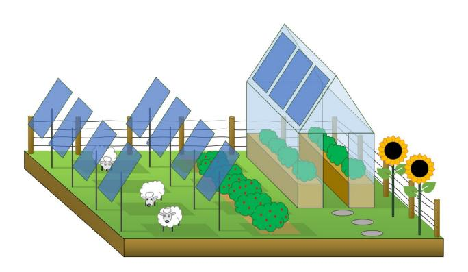
An illustration showing three applications of agrivoltaics. A protected cropping environment, such as an advanced greenhouse (right), in which lightweight, semitransparent PV cells are integrated into the roof and/or walls. Semitransparent PVs and opaque PVs can also be combined with open cropping environments and livestock, providing shade while also generating power (left). Credit: Austin Kay
