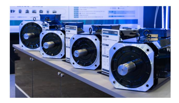
Spindle motor, a component of KERI's 'CNC Drive System' Credit: Korea Electrotechnology Research Institute (KERI)
