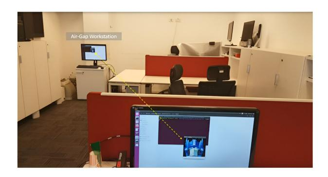
Attack demonstration. An air-gap workstation processes a secret image (Optimus Prime). The RAMBO covert channel attack transmits the image via electromagnetic waves. A remote attacker intercepts the information and recovers the secret image. Credit: *arXiv* (2024). DOI: 10.48550/arxiv.2409.02292
