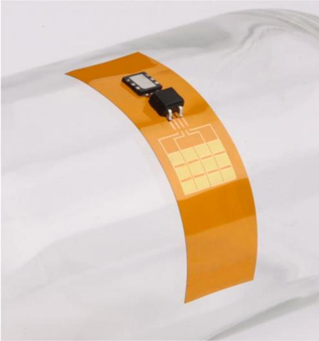
Thin, flexible mechanical energy harvester, with rectifier and microbattery, mounted on a curved glass support. Credit: University of Illinois and University of Arizona.
