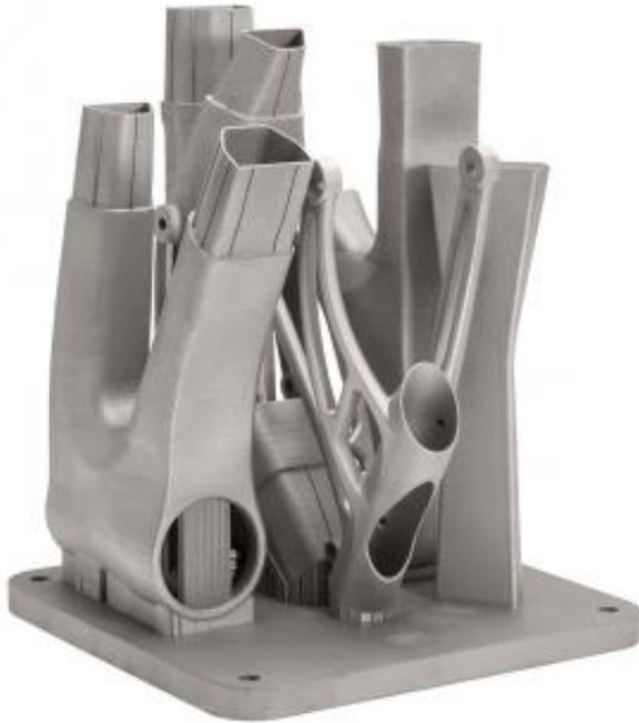
The entire bike frame was arranged in sections with the seat post bracket on one build plate and fabricated in one go
