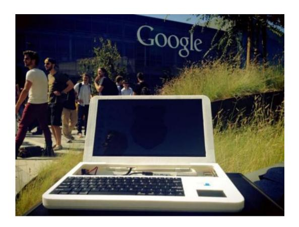
Using PLA filament, a small London-based team have managed to achieve the 3D printing of their own Raspberry-Pi-based laptop, with a battery life of six to eight hours and Wi-Fi enabled out of the box. They are offering it to others in the form of a kit that they will bring to Kickstarter. Namely, they will offer a Raspberry Pi- powered laptop kit
