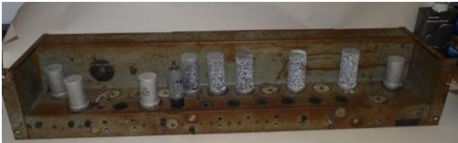
Chassis 1A, a Storage Regeneration Unit that keeps data recirculating through a short or long tank. Credit: The National Museum of Computing
