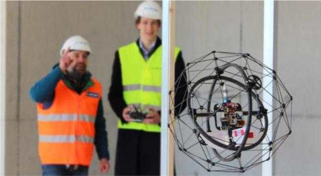
Flyability drones are going to advance a perception of drones as service angels as opposed to attack agents. Switzerland-based Flyability is all about making robots to support search and rescue operations. Their product is a small, lightweight drone which can collide on obstacles without losing stability and is safe to fly in contact with humans.
