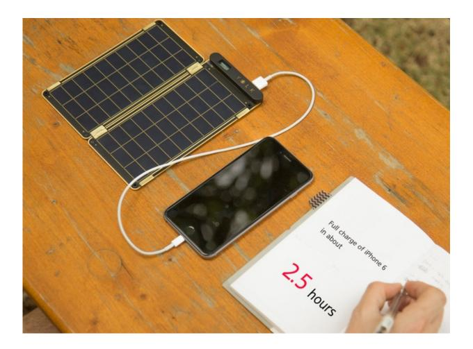
For example, tablet PCs that require more power can be charged by adding additional panels—magnet connectors help to add or subtract the solar panels. ("The basic 5 watt Solar Paper can charge your smartphone on a sunny day. If you need more power to charge a tablet, or to charge on a cloudy day, you can click new magnetic panels into place," the campaign page stated.)
