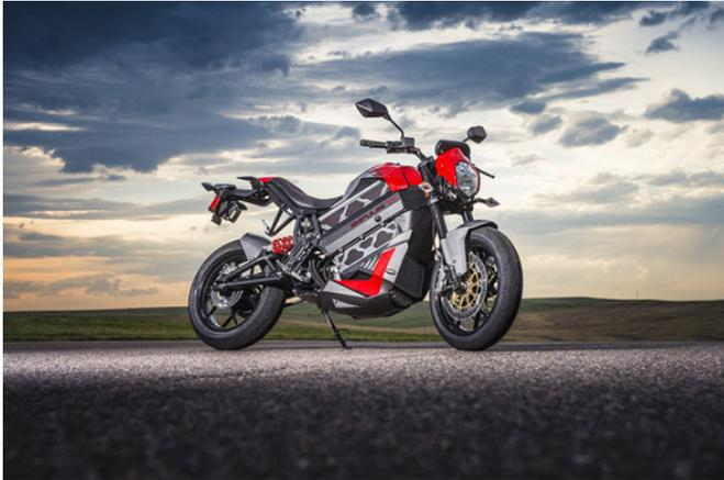
Victory Motorcycles has introduced its Empulse TT, the first all-electric addition to the Victory lineup. Features include adjustable suspension featuring a single rear shock and inverted front forks; dual-disk front brakes for high-performance stopping power; lightweight aluminum wheels; and an LCD instrument display.
