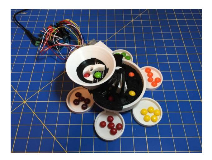
A 3D-printed Skittles sorting machine that can sort the colors into bins is
